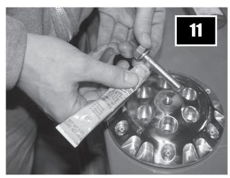
**11.** Install the clutch adjusting screw using a small amount of high temp grease or antisieze on the threads & on the clutch pushrod end.
