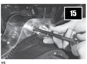
15. Install the starter jackshaft cover using blue thread locker on the bolts.
