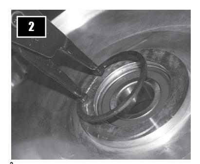
2. Install the appropriate supplied motor plate bearing & circlip for your application into the motor plate. 07-earler / 08-later models use different bearings.
