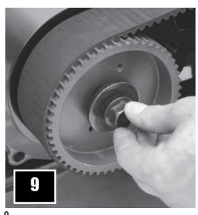
Install & torque the OEM compensator bolt to manufacturers specs. Always clean bolt thoroughly and apply red thread locker before installing.
