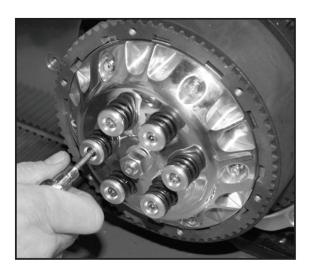
After installing pressure plate, install clutch springs w/supplied spring collars and narrow-headed 12-24 bolts. Install using Blue Locktite. Spring collars should bottom on clutch hub studs. Torque to 90 in-lbs. In higher horsepower applications, heavier springs are available.
