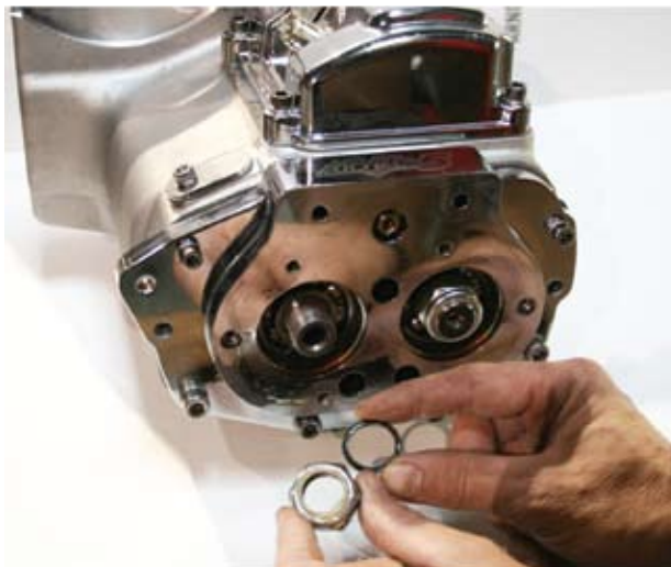
Remove the mainshaft nut. 5 speed models will have an additional spacer behind the mainshaft nut. This spacer will also need to be removed. These will not be reused.
