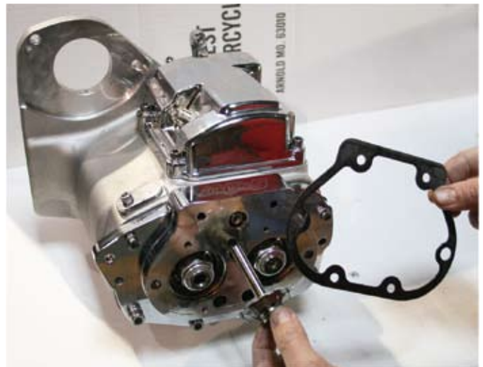
Remove the stock clutch throwout assembly & gasket. These will not be reused.
