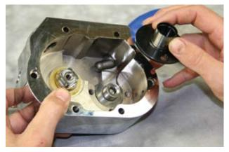
Remove the three ½-20 flathead bolts from the mainshaft gear guide & then remove the gear guide.
