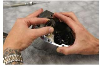
Remove the 2 thrust washers & the center bearing assembly. Note that there is a thin & thick thrust washer. The thin thrust washer will be on the bottom.
