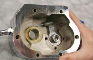
Verify that the Oring is installed onto your clutch cable then install your clutch cable. Tighten your clutch cable to the kicker cover using a 9/16 wrench. Do not overtighten.
