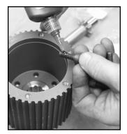
I. Ultima Drives use 6 bolts to fasten the motor pulley to the pulley insert. Install these bolts using red Loctite and tighten to 18-22 ft lb torque.
