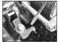
Check your kickstand clearance to the belt by pushing down on the belt then adding at least 1/2".
