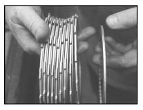
Ultima<sup>®</sup> 3.35" belt drives utilize 9 of the old style 900cc Sportster<sup>®</sup> steel drive plates and 9 special size fiber plates designed to provide a very adjustable clutch package. When Installing the clutch pack, install the thick .119" steel plate first, then alternate fiber/steel. The last plate you install should be fiber.
