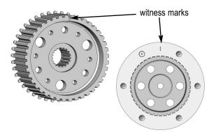
3. Align the witness marks on the pressure plate and inner clutch hub as shown when assembling.
