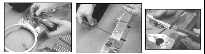
3. Using red Loctite Install the remaining 5 long outer cover spacers with set screws into the motor plate. Motor plates are drilled through so you can access the allen head from the inside. Put the hex side of the set screw into the motor plate. Use red Loctite on outer cover spacers
