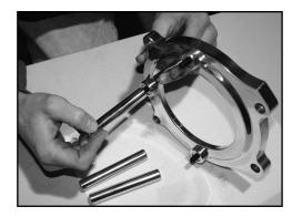
2. Install the 3 shorter outer cover spacers using red Loctite & the supplied set screws. Motor sub plates are drilled through so you can access the allen head side of set screw from the inside.
