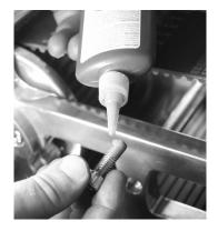
After all pulley caps are tight, reinstall the outer support plate using blue Loctite. Torgue bolts to 15-18ft lb.
