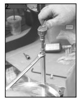
4. A good way to tighten the outer cover spacers is to use one of your 5/16-18 bolts and a jam nut. This will allow you to get some torque on the spacers.
