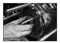
2. Install the stator, rotor, washer and any shims that were present or are needed. (see notes concerning stock pulley insert if utilizing the provided insert)
