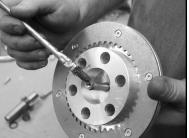
2. Check the pressure plate screws to ensure they are all tight and the heads of the bolts are sitting below the plate surface. Install the clutch adjusting screw using a small amount of high temp grease on the thread and especially on the clutch pushrod end. Don't get to much grease out there –Remember this is a DRY clutch.
