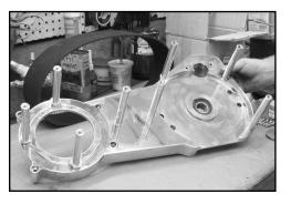
5. The motor plate and motor sub-plate ready for assembly.
