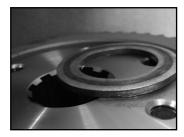
3. When using a stock offset spacer/insert, always use the proper thickness shim between the pulley and the rotor. Failure to do so will result in improper torque on the outer portion of the motor pulley instead of the pulley insert.
