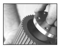
All Ultima Drives include the stock offset spacer/insert. For wide tire applications see list below for proper pulley insert/spacer
