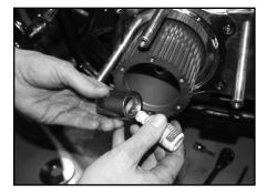
3. Install the motor pulley nut using red Loctite and torque to mfg recommended specification.
