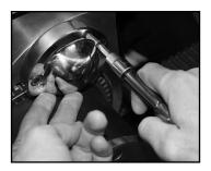
6. Install your starter motor to the motor plate, then install the starter drive gear assembly in the order shown using blue Loctite. The starter drive gear should be a minimum of .150" from the clutch basket starter ring gear once installed. APPLY SOME HIGH TEMP GREASE TO THE STARTER END CAP BUSHING. Apply upward pressure to end cap when torquing to 18-22 ft/lbs. Always use blue Loctite on end cap bolts. Reapply grease to bushing every 6 months minimum - DO NOT RUN DRY!
