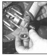
I. Install the clutch basket assembly onto the transmission mainshaft. Apply red Loctite to the mainshaft nut and torque to 55-65 ft lb.
