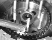
4. Check the inner stud alignment using the clutch spring collar flipped over with the flange side in. The collar should pass through the pressure plate freely a minimum of 1/4". Straightening is generally not required, but if needed, straighten the stud by using a small brass drift.
