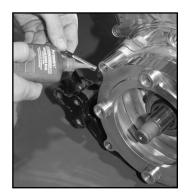
**3.** Install the motor plate and motor sub-plate without the rubber o-ring for the inner primary to engine. Align the motor plate to the engine and transmission then install the mounting bolts for the engine and trans snug only. You might need a dead blow or plastic hammer to seat the motor plate over the transmissions dowel pin. Using red Loctite, torque all bolts to 18-22ft lb.
