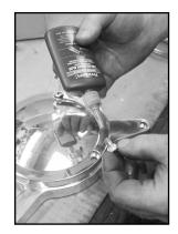
Install outer cover caps onto the outer cover using blue Loctite. Torque to 18-22 ft lb. Note the bolt clearance notch location on the motor pulley cap to the outer plate.
