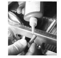
2. After all Pulley Caps are tight reinstall the outer support plate using Blue Loctite. Torque Bolt to 15-18ft lb.
