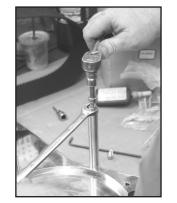
4. A good way to tighten the outer cover spacers is to use on of your 5/16-18 bolts and a Jam Nut. This will allow you to get some torque on the spacers.
