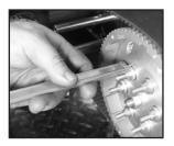
5. Install the clutch springs and clutch spring guides with the flanges out. Install the Clutch Spring nuts until you measure .350"+/- .010 from the face of the pressure plate to the face of the spring guide as shown. This sets the Spring at approx. 1.250 installed height. For higher power applications go in to .100" measured max for 1.000 installed height. Ultima Belt Drives come with a standard pressure spring for most applications under 100 hp.
