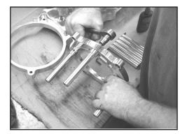
2. Install the 3 shorter outer cover spacers #56B into the Motor Sub-Plate # 5 using Hardware # 66 Black Oxide finish with Red Loctite. Torque to 18-22 ft lb
