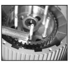
**4.** Check the Inner Stud Alignment using the clutch spring collar flipped over with the flange side in. The Collar should pass through the pressure plate freely a minimum of 1/4". Straightening is generally not required but if needed straighten the stud by using a small brass drift.
