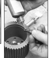
Ultima Drives use 6 bolts to fasten the Motor Pullev to the Pullev Insert. Install these bolts using Red Loctite and Tighten to 18-22 ft Ib torque. All Ultima Drives include the Stock offset Spacer. The Following Spacers are available separately for Wide Tire Applications.
