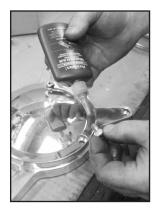
6. Install Outer Cover Caps onto the Outer Cover using Blue Loctite. Torque to 18-22 ft lb. Note the bolt clearance notch location on the motor pulley cap to the outer plate.
