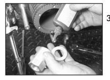
Install the motor pulley nut using RED Loctite and Torque to Mfg recommended Specification.
