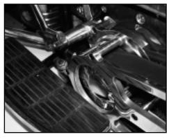
Ultima 2" Bagger Belt Drives are designed to work with stock floorboards. We recommend verifying there are no clearance issues w/your floorboards at this time. Shim/space as necessary.
