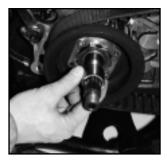
Before installing the motor plate you must remove the inner primary race from the transmission mainshaft if it is present.
