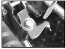
Check your kickstand clearance to the belt by pushing down on the belt then adding at lease 1/2' of travel. Use MWM # 5-190 adjustable kickstand leg stop if needed. This is an important safety check and should be performed before initial startup.
