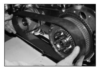
Ultima Belt Drives are not as sensitive as chain drives to pulley alignment as the clutch basket acts as a guide but proper alignment should be checked. To insure a completely dry running primary many people use a bead of clear RTV Silicone at each spline to insure no oil will travel between the shaft and spline.
