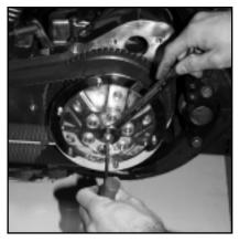
At this time you will adjust your clutch. Thread in the adjuster until it makes contact w/the clutch pushrod. Once it is lightly seated, back adjuster off 1/4 turn. Using an 11/16" wrench, tighten the adjuster locknut. Clutch cable adjustment can now be done leaving some end play at the lever.
