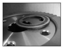
Ultima Drives use 6 bolts to fasten the motor pulley to the pulley insert. Install these bolts using red Loctite and tighten to 18-22 ft lb torque. All Ultima Drives include the stock offset spacer. When using a stock offset spacer, always use the proper thickness shim between the pulley and the rotor. Failure to do so will result in improper torque on the outer portion of the motor pulley instead of the pulley insert.
