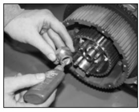
Install the clutch basket assembly onto the transmission mainshaft. Apply red Loctite to the mainshaft nut and torque to 55-65 ft lb.
