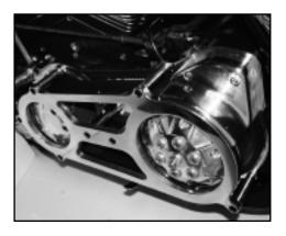
Install belt covers using the supplied spacers, hardware & blue loctite. Torque bolts to 18-22 ft lbs.
