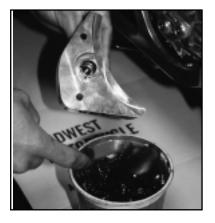
Install your starter motor to the motor plate then install the starter drive gear assembly in the order shown using blue Loctite. The starter drive gear should be a minimum of .150" from the clutch basket starter ring gear once installed. **APPLY SOME HIGH TEMP GREASE OR ANTI-SIEZE TO THE STARTER END CAP BUSHING.** Apply upward pressure to end cap when torquing to 18-22ft lbs, always use blue Locktite on end cap bolts. Reapply grease to bushing every 6 months minimum - **DO NOT RUN DRY!**
