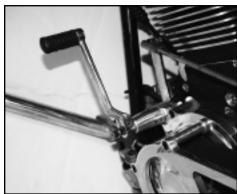
Before installing the shifter assembly we recommend lubricating the shifter bushing & shaft for smoother & quieter shifting operation. Install shifter, spacers & shims as shown in the picture.
