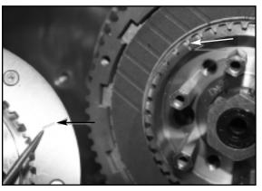
Align the witness marks on the pressure plate and inner clutch hub as shown when installing pressure plate. This will insure clutch hub studs will be centered in the appropriate pressure plate holes.
