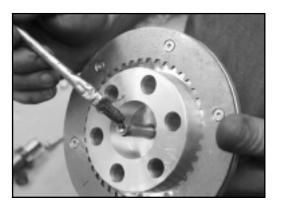
Ultima 2" belt drives utilize 8 of the old style 900cc sportster steel drive plates and 8 special size fiber plates designed to provide a very adjustable clutch package. When installing the clutch pack install the thick .119" steel plate first then alternate fiber/steel. The last plate you install should be fiber.
