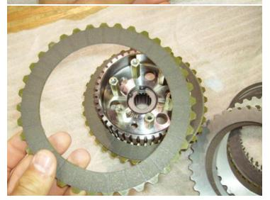
You will end with an outside splined plate with the friction side out. This friction side will then contact the steel surface attached to the pressure plate.
