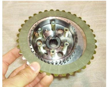
Install the inside splined plate (note—one side is steel the other is friction). Installing in this manner will mean that from here on all steel sides will go in and friction sides will go out.
