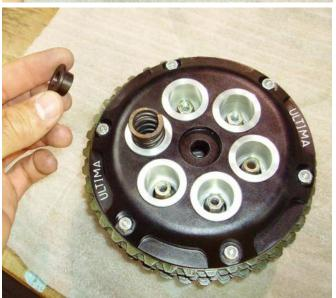
Install all six bolts. These bolts will tighten until they are bottomed leaving the correct amount of space for pressure plate movement
