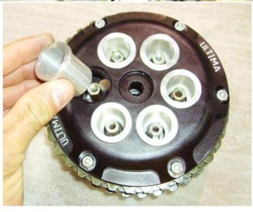
Next install all six springs. Three spring rates are included for you to choose your strength. Higher the spring rate the more horsepower the clutch will hold.
