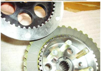
Next install the spring cups. These will just slide into place as long as the markings (shown above) are aligned.
