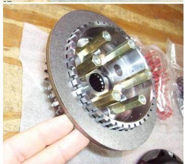
Install the double sided friction plate next. There is only one of these plates per kit.
