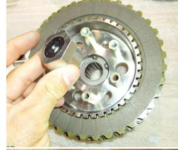
Step TWO: Installing the clutch plates; Install the thick steel first.
