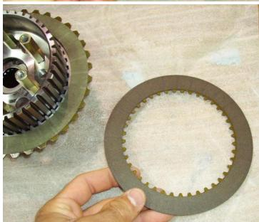
Install the outside splined plate next and repeat the pattern (inside spline, outside spline)
