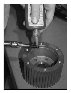
Ultima Drives use 6 bolts to fasten the Motor Pulley to the Pulley Insert. Install these bolts using Red Loctite and Tighten to 18-22 ft lb torque. All Ultima Drives include the Stock offset Spacer. The Following Spacers are available separately for Wide Tire Applications.
