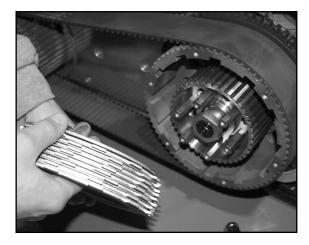
1. Ultima Belt Drive utilize 8 of the old style 900cc sportster steel drive plates and 8 special size fiber plates designed to provide a very adjustable Clutch Package. When Installing the Clutch Pack Install the Thick .119" Steel Plate First then Alternate Fiber/Steel. The Last Plate you install should be Fiber.
