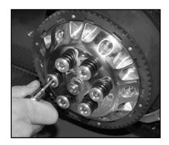
5. After installing pressure plate, install clutch springs w/supplied spring collars and narrow-headed 12-24 bolts. Install using Blue Locktite. Spring collars should bottom on clutch hub studs. Torque to 90 in-lbs. In higher horsepower applications, heavier springs are available.
