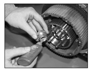
1. Install the clutch Basket Assembly onto the transmission mainshaft. Apply RED Loctite to the mainshaft nut and torque to 55-65 ft lb.
