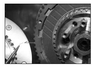
**4.** Align the witness marks on the pressure plate and inner clutch hub as shown when installing pressure plate. This will ensure clutch hub studs will be centered in the appropriate pressure plate holes.
