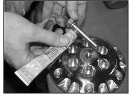
3. Install the clutch adjusting screw using a small amount of high temp grease or anti-sieze on the thread and especially on the Clutch Pushrod end. Don't get too much grease out there –Remember this is a DRY clutch.
