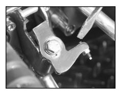
Check your kickstand clearance to the belt pushing down on the belt then adding at lease 1/2". Use MWM # 5-190 Adjustable Kickstand Leg Stop if needed. This is an important safety check and should be performed before initial startup.
