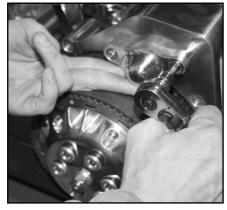
Install your starter motor to the Motor Plate then install the starter drive gear assembly in the order shown using Blue Loctite. The Starter Drive Gear should be a Minimum of .150" from the clutch basket starter ring gear once installed. **APPLY SOME HIGH TEMP GREASE OR ANTI-SIEZE TO THE STARTER END CAP BUSHING.** Apply upward pressure to end cap when torquing to 18-22ft lbs, always use Blue Locktite on end cap bolts. Reapply grease to bushing every 6 months - **DO NOT RUN DRY!**
