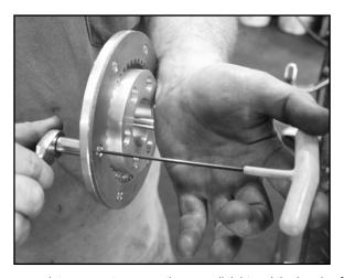
2. Check the pressure plate screws to ensure they are all tight and the heads of the bolts are sitting below the plate surface.
